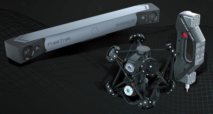
Portable Wireless Optical Coordinate Measuring System:
